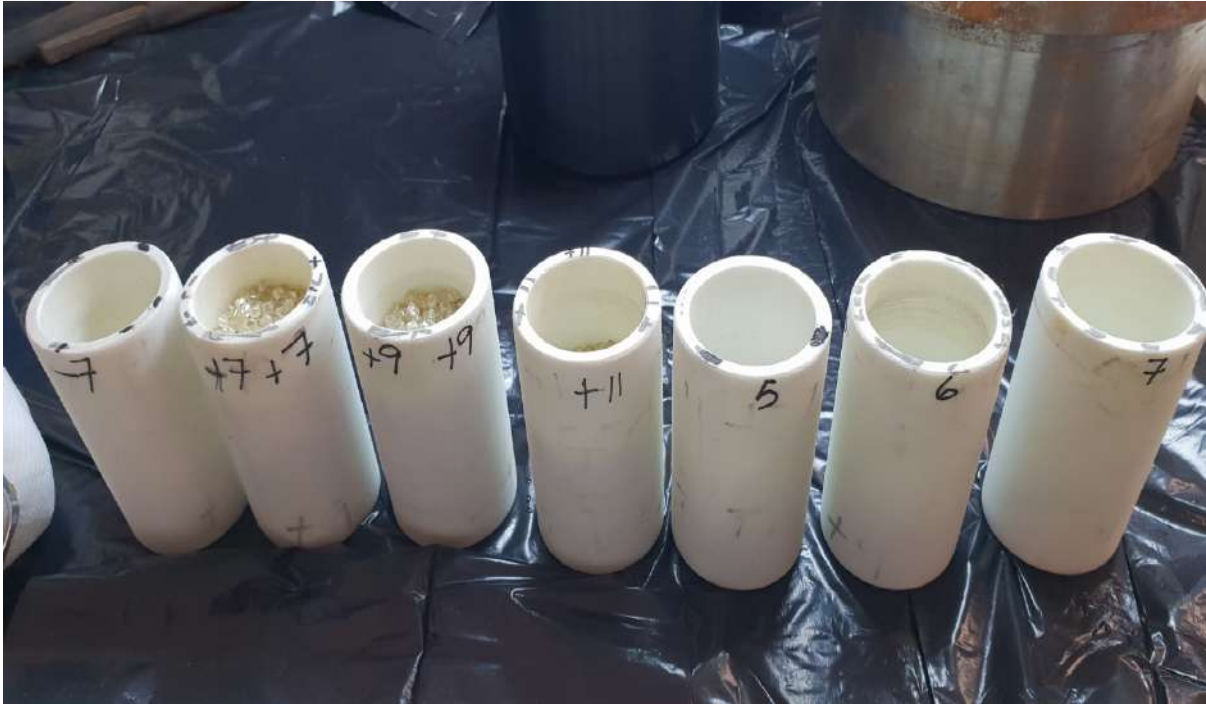
Figure 4: Ceramic pots containing diamonds for acid cleaning
