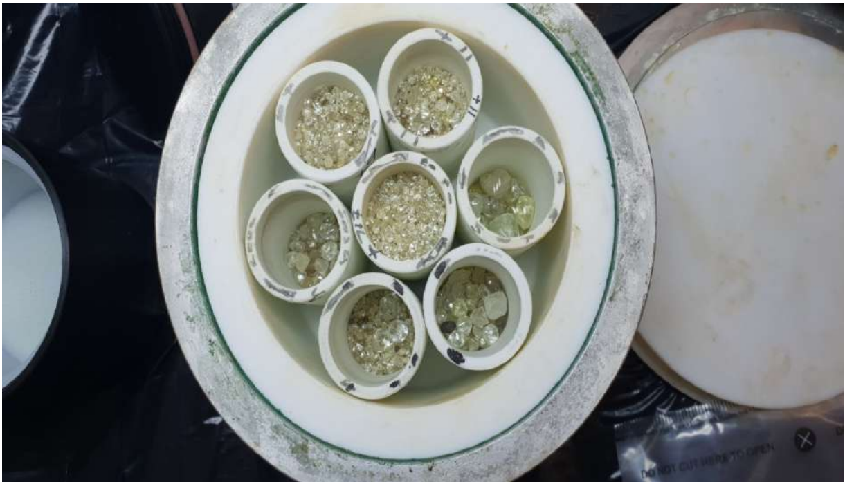
Figure 5: Ceramic pots placed into a ceramic vessel for pouring of the acid
